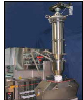
Zig-Zag Flour Reclaim System
