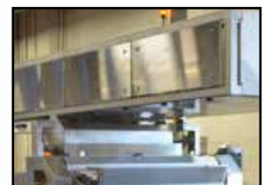
Stainless Steel Side Panels and Hinged Catch Pans
