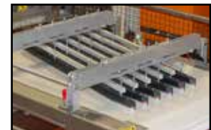
Hinged Rounder Bars with Gas Spring Assist
