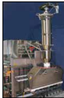
Zig-Zag Flour Reclaim System
