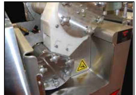
Accurate Sliding Vane Style Metering Pump and Gentle Single Auger Design
