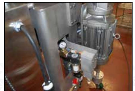
Slide out Access Panel to Access Vacuum Generator
