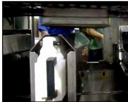
High efficiency AMF Air Knife removes leftover crumbs.
