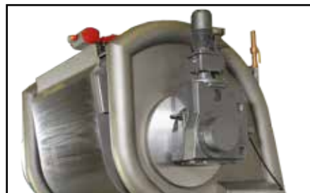
Maintenance-free Direct Drive Tilt Mechanism
