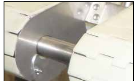
Two-Piece Safety Sprocket Guard
