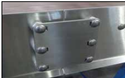
Junction Plate Stands Off For Efficient Sanitation
