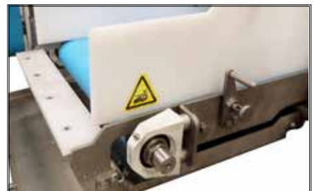
Removable Scraper - No Tools Required
