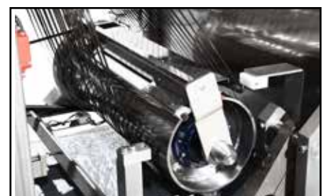
Cantilever Drum Design for Easy Blade Removal & Replacement
