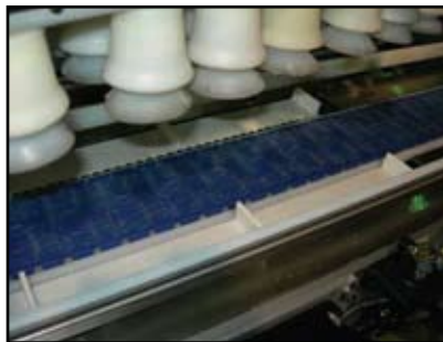
Flighted Timing Belt for Indexing Brown 'n Serve Boxes
