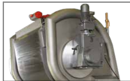
Maintenance-free Direct Drive Tilt Mechanism
