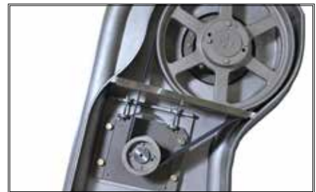
Main Agitator Drive Side
