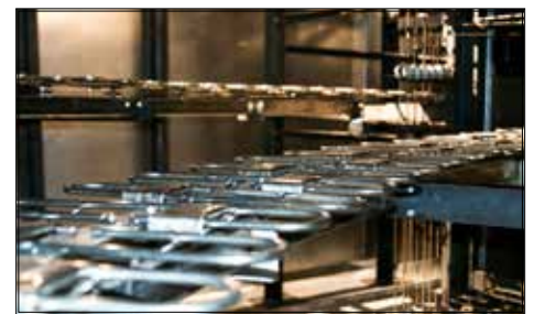
Sealed, Bolted Track Curves
