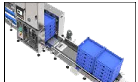
Stack Feed System
