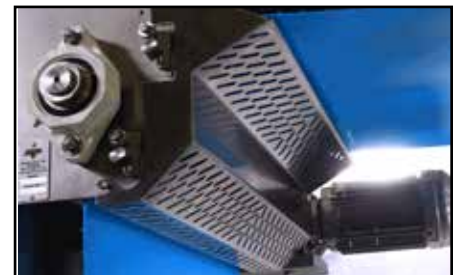
Toolless Guard Removal
