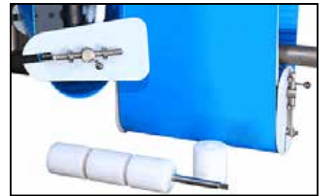
Easily Removable Idler Roller
