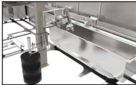
Trough Oiling Station
