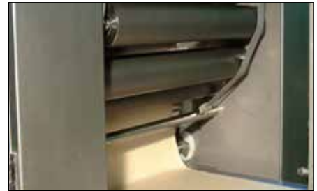
Multi Roller Reduction Station
