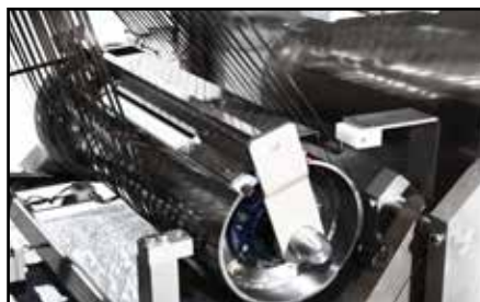
Cantilever Drum Design for Easy Blade Removal & Replacement
