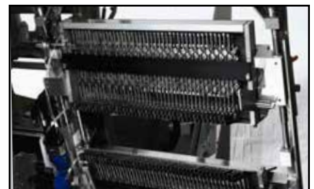
Heavy Duty Self Supporting Stainless Steel Lattice Pull-out Mechanism
