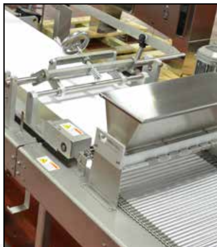
Motorized Dough Guide Adjustment with Digital Readout
