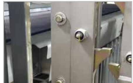
Laser-Cut Greaseable Pawls
