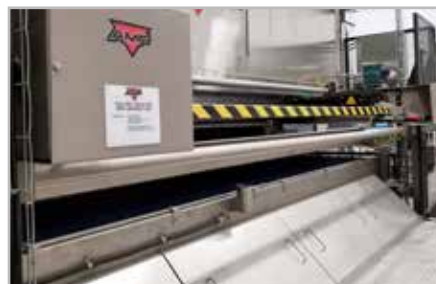
ST-ST Panel Guards Cover Front Pit
