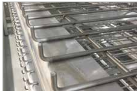
ST-ST Grid Rods 90° Bent Up & Down
