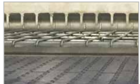
Laser-Cut Interference-Free Pusher Fingers
