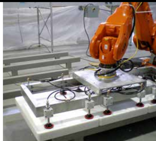
PEEL BOARD STACKING & UNSTACKING SYSTEMS
