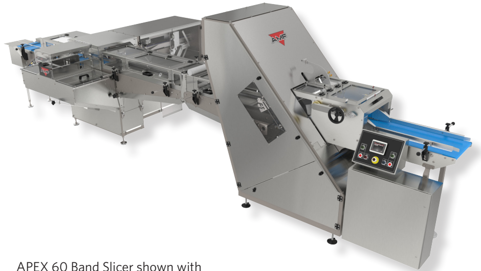
APEX 60 Band Slicer shown with optional infeed extension integrated to APEX 60 Bread Bagger
