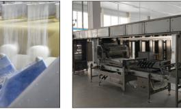
Direct drive intermediate proofer tower with single action flapper gate to control the drop from the proofer to the sheeter for accurate dough ball placement.
