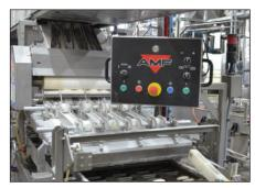
Adjustable 6" (152 mm) diameter steel, non-stick sheeter rollers provide precise sheeting and timing. Declined moulder section relieves pan jams and improves panning accuracy.
