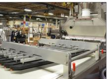
Poly-slick, direct-drive rounder belt and patented spiral tunnel rounder bars provide excellent rounding without dough stickage for simple cleaning.
