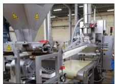
Stainless steel Accumax or RollFlex Extrusion Divider frame, hopper, feed screw, and developer ensure durability and minimum flow resistance.
