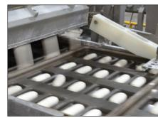
Rotary action mechanical pan indexer for smooth pan indexing and quick change index bars for easy product changeover.
