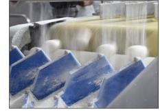
Pneumatically actuated flour sifter with individual lane blockouts, flapper gate, and flour catch pan with return port for flour recovery integration.
