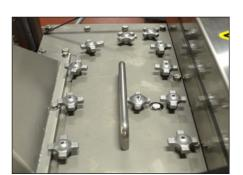
Patented 'quick-clean' dough manifold system with precise flow control diverters and quick clean access for reduced sanitation costs.
