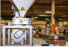
Built-in DoFlow degassing system supplies consistent, uniform dough density.
