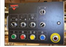
Simple Allen-Bradley operator control station located on the proofer tower with recipe management of 30 products.
