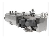
Close-coupled, independent VFD drives eliminate high maintenance chain and sprocket sequence drives that traditionally run the length of the machine.
