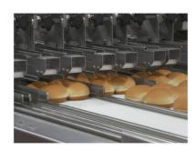
For maximum flexibility, the high speed system manages 8 to 10 individually adjustable lanes to accomodate varying sized products.
