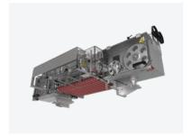
Single band slicer is available to cut buns horizontally in a single, uniform cut slicing buns in half. A dual band slicer option is available utilizing two blades to create two parallel cuts in a single pass.
