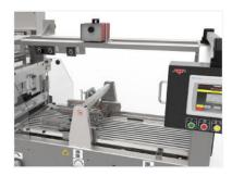
A low profile, ergonomic frame design improves the operator experience with a conveniently placed menu-driven control panel and easy access safety guarding.
