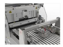
Impulse cross seal and cut system provides the strongest seal available with precision temperature control while eliminating the high maintenance seal bars and knife for outstanding seal quality.
